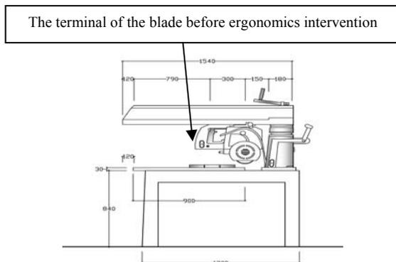
Figure 1 The Radial Saw Machine Before Redesign of Work Station
