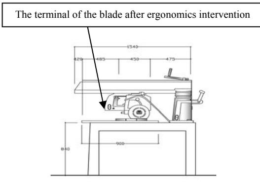
Figure 2 The Radial Saw Machine After Redesign of Work Station
